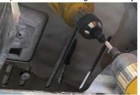
6. Insert next 3 screws as shown. Don't forget lock washers. Leave loose for now. Final check on winglet position before inserting last screw with lock washer.
