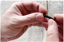
7. Insert screw through center hole in wicker bill and into center rivet nut, but don't fully tighten with 1/8" hex bit or Allen wrench.
