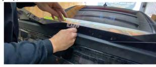
15. Top 2 gurney flap holes use 1/2" screws, recessed washers and nylock nuts. Fully tighten with 1/8" hex bit or Allen wrench and 3/8" socket or wrench
