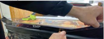
13. With 3/4" screw inserted through recessed washer and center hole of gurney flap, screw into center hole of wicker bill.
