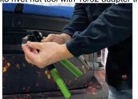
5. Squeeze rivet nut tool firmly to the point you feel it stop then slightly more to ensure tight fit of rivet nut. Be careful to not strip rivet nut. Unscrew rivet nut tool from rivet nut.
