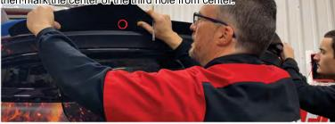
9. Remove wicker bill. Drill out hole making sure you center drill bit on marks you made in the center of wicker bill hole. Remove tape around
