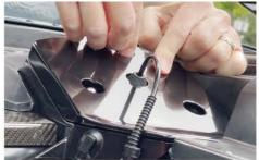
8. Reconnect Mag-Ride Wire After Ensuring the Connectors are Properly Oriented
