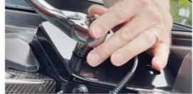
9. Reattach Connectors to Strut Tower by Aligning Groove on Connector to Holding Tab on Strut Tower and Sliding Up Until Locks in Place
