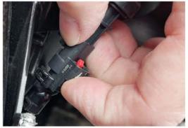
3. Press Tab Towards Rear of Car to Release Connector and Slide Down
