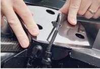
7. Using a 13mm Socket and Wrench, Tighten Acorn Nuts. Do Not Over Tighten (Non-Mag-Ride Repeat for Other Side and Done).
