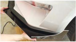
8. Make Sure Splitter Side Section is Straight with Stock Splitter and Still in Desired Location. Tighten Remaining Existing Screws. Repeat for Other Side.
