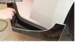
10. Install 21 Pointed Screws with Silver Lock Washers into Small Holes in Air Splitter Sections. If Using Power Tool, Don't Fully Tighten. Go Back and Hand Tighten to Avoid Over Tightening and Stripping Out Plastic.
