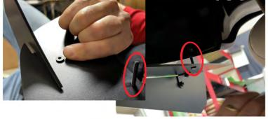
14. For regular body Challengers, the area of plastic for this screw is small so take extra care to get screw into plastic without going over edges while also trying to keep screw hidden from view from the side of the car. For wide bodies, be sure that the middle screw hole from step 15 is in a good position and placement of side blade holder in relation to outside edge of bumper is to your liking before you install this screw. Do not fully tighten yet.
