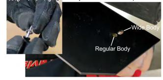
15. Take another shorter install screw and external star washer and install it in the L-bracket hole as shown. Do not fully tighten yet.
