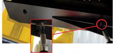
17. Go back and hand tighten all mounting screws being careful to not over tighten and strip out bumper plastic. Double check that all is secure before driving.
