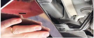
11. Diffuser is slotted so you can adjust how far out you want the diffuser. Once diffuser is in place, tighten silver screws with 1/4" wrench and ensure diffuser remains straight and at the distance from the car you desire.
