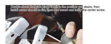
Periodically check all screws to ensure they remain tight. ONLY TIGHTEN AGAIN IF LOOSE. Do not over tighten when installing screws into stock diffuser. If screw strips out of plastic, use a larger screw or a bolt and nut and do not drive with diffuser installed until fixed. EMP is not responsible for products beyond initial quality and condition due to conditions, installation quality and other factors beyond our control.
