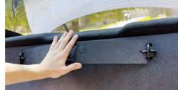
15. Use seat back center hinge bolt removed earlier to secure center hole to car. Leave loose so you can adjust fit for other holes.
