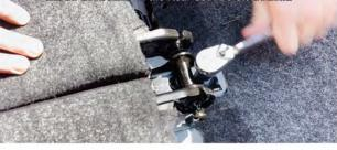
10. Pull seat back side hinge straight up off of bolt and remove from car Hinge Bolt Repeat for other side 3. Pull on seat bottom to disengage from spring and hinge. May need to move fabric to clear spring and hinge and keep from tearing.
