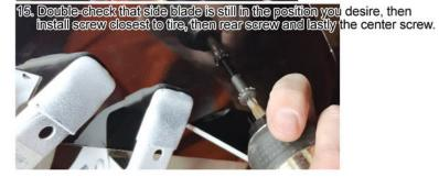
Hand (tighten all side blade mounting screws. Be sure to not over tighten and strip out side rocker plastic. Repeat full side blade process for other side blade.
