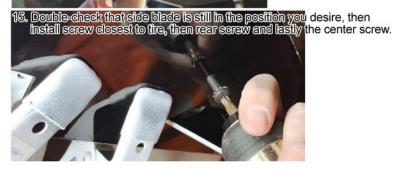
Hand (tighten all side blade mounting screws. Be sure to not over tighten and strip out side rocker plastic. Repeat full side blade process for other side blade.
