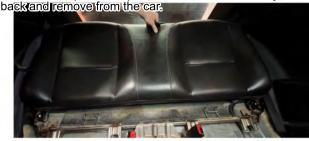
8. SEAT DELETE INSTALL: Bring seat delete back section into car
