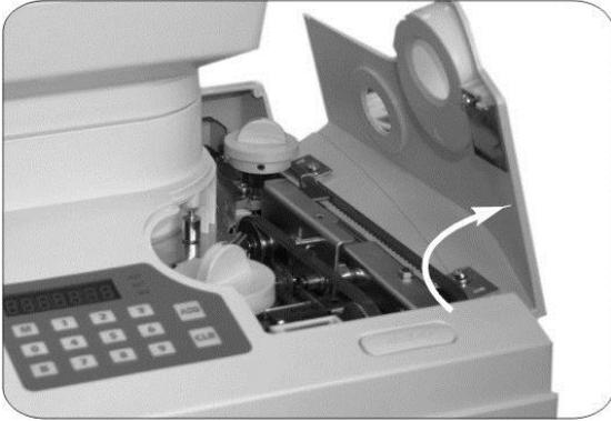
Then, pull up the Front Feed Pulley Arm and push & pull the Lock Plate upward to remove the foreign objects.
