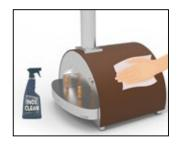
**5. Protect stainless steel.** To better protect the stainless steel parts, we suggest using vaseline oil or other neutral cleaning solutions (pH 7) that do not contain acids, white spirit or xylene. Use soft, non-abrasive cloth to apply. In the case of beachfront installations to avoid salty air corrosion and white thin layers, clean the oven often with fresh water.
