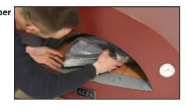
**3** - Remove the laser protective film from all stainless steel parts, such as: sill, door, flue and chimney. Use a hair dryer to speed up the procedure and easily remove the laser film.
