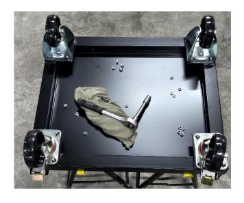
4 - Insert the long screws with the nuts to another side and tighten well.
