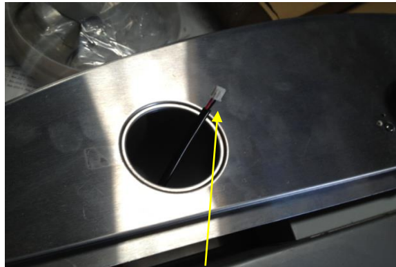
Figure 16: Connect All Wires to the LED Lights
