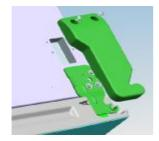
2. Screw off the three bolts fixing the upper hinge, remove the upper hinge, and pry off the door shaft sleeve, magnet and the proximity switch on the upper hinge cover.
