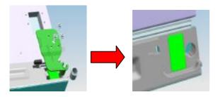
3. Screw off the three bolts fixing the top box cover on the left side, remove the box cover, take the wire harness out
