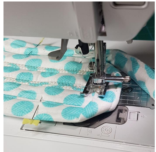
Figure 10 Continue stitching and rotating the spiral, removing the pins as you go.
