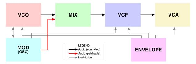
Using the same color-coding, the following illustration shows the location of these modules (and their corresponding patch points) on Atlantis' front panel:
