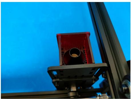
Figure 35. Laser aperture of model A5 30W
