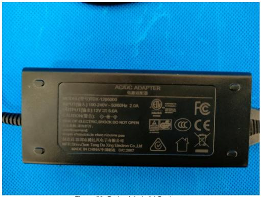
Figure 53. Rating label of AC adapter
