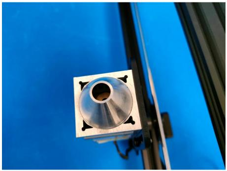
Figure 22. Laser aperture of model A5 50W
