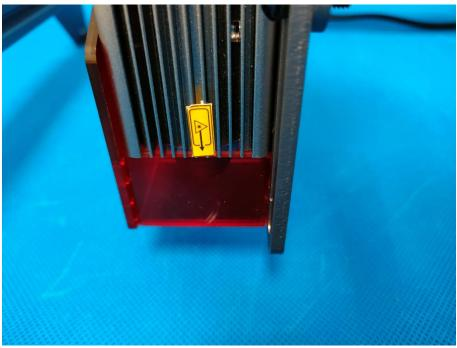
Figure 28. Laser aperture marking of model A5 Pro 40W
