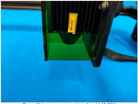
Figure 49. Laser aperture marking of model A5 20W
