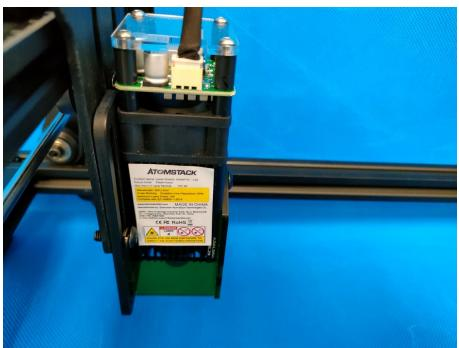
Figure 48. Laser label of model A5 20W
