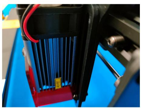
Figure 42. Laser aperture marking of model A5 40W
