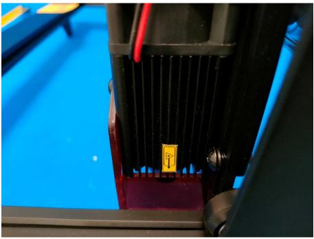
Figure 36. Laser aperture marking of model A5 30W
