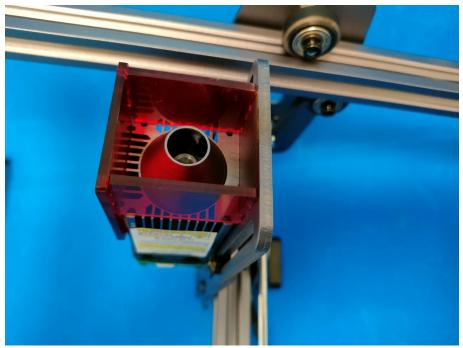
Figure 29. Laser aperture of model A5 Pro 40W
