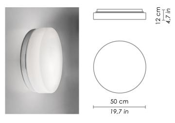
Wall-ceiling lamps with diffuser in mouth-blown, satin-finish opal triplex glass; chlorine-resistant, anti-UV, neutral translucent polycarbonate frame, with chrome or matt white painted metal parts. Twist-lock coupling system f or the glass component. The product is suitable for indoor use only. Drum Metal is IP44.
