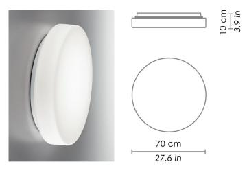
Wall-ceiling lamps with diffuser in mouth-blown, satin-finish opal triplex glass, and white painted metal frame. Twist-lock system for the glass component. The product is suitable for indoor use only.
