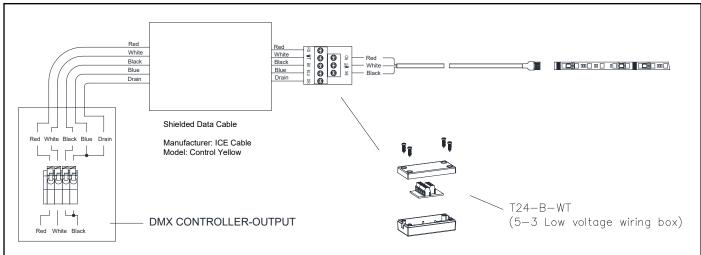
**Option B:** LUTRON -16/2 or 18/2 Stranded, and 22/2 Stranded Shielded Cable Manufacturer: Lutron
