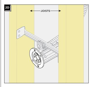
Cut a 2.75" diameter size hole and install drywall to the joists.
