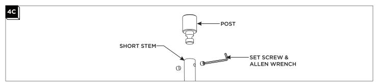
6 Remove the set screws around the short stems and remove the post from each stem. Set the set screws aside for later in the installation.
