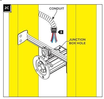
Attach conduit to either the top hole or the back plate of the junction box. Run low-voltage wires from the transformers into the junction box.
