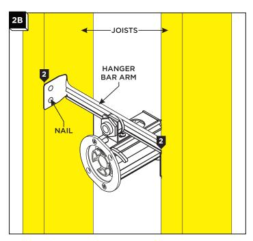
2 Extend hangar bar arms to the left and right joists and nail into place.
