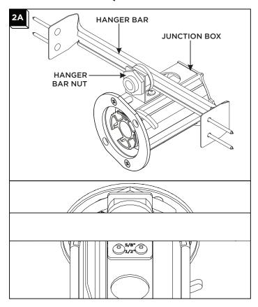
Use the markings on the bracket according to your wall thickness. Choose between 0.5" or 0.625" thick walls. Place the hanger bar on the bracket and secure the together using the hanger bar nut.
