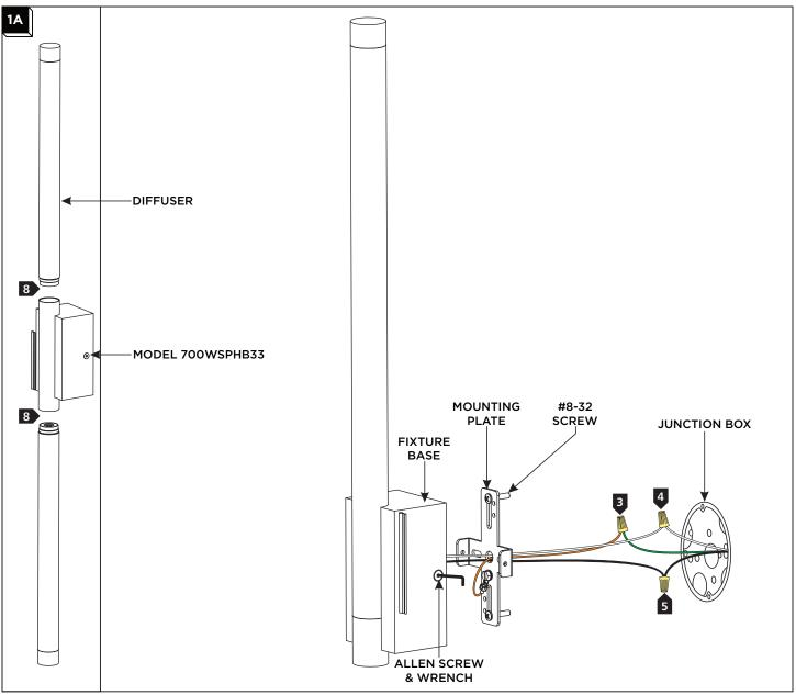
1 With the provided Allen wrench, loosen (do not remove) the set screw on the fixture base.
