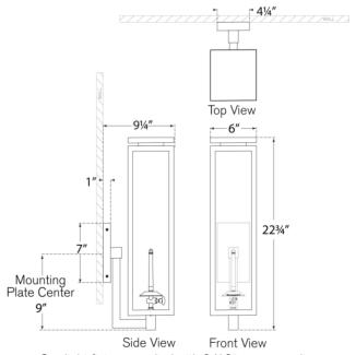
Gas light fixture supplied with 3/16"copper gas line and 3/16" x 1/4" gas line adaptor
