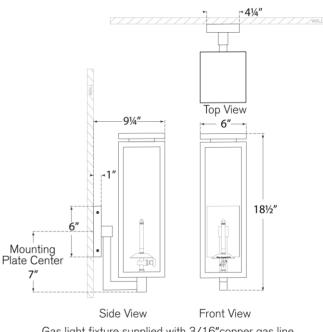
Gas light fixture supplied with 3/16" copper gas line and 3/16" x 1/4" gas line adaptor
