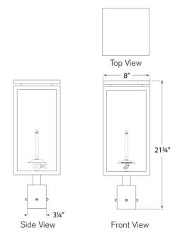
Gas light fixture supplied with 3/16" copper gas line and 3/16" x 1/4" gas line adaptor
