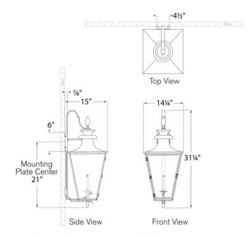
Gas light fixture supplied with 3/16" copper gas line and 3/16" x 1/4" gas line adaptor
