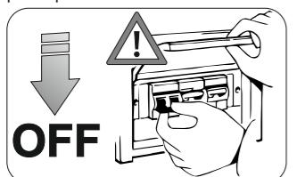
**BEWARE:** Connecting the fitting when power is on could irremediably damage the LEDs.
