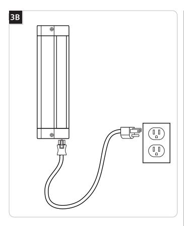
Using the Plug-In Wall Feed, plug the Undercabinet unit directly into a wall outlet.
