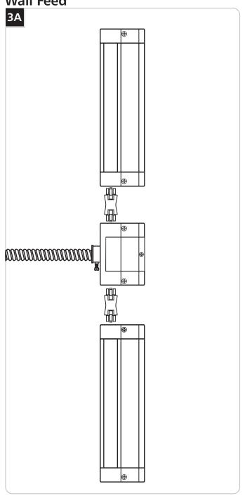
Using the jumper connectors, link Undercabinet units to either or both ends of the Splice Box.
