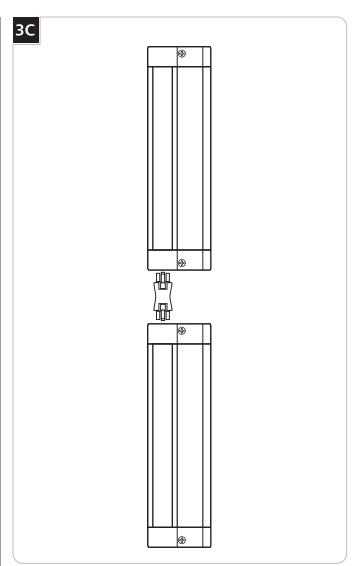
Remove the connector cover and use the Jumper Connectors to link multiple Undercabinet units to one another.
