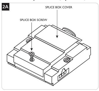
1 Loosen the center screw on the splice box and remove the cover.
