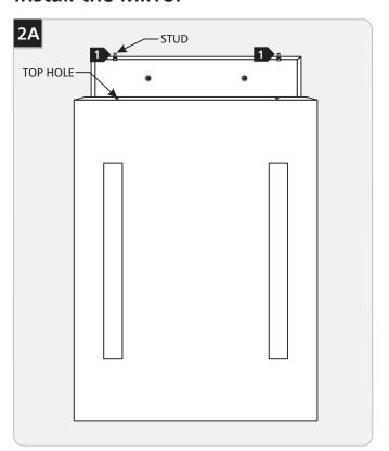
1 Carefully hook the mirror through the top two holes onto the backplate studs.
