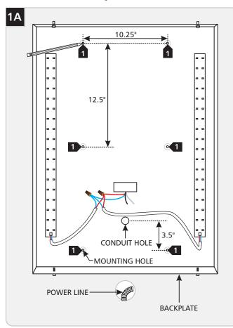
NOTE: This installation requires an additional person to hold the backplate while electrician installs it.
