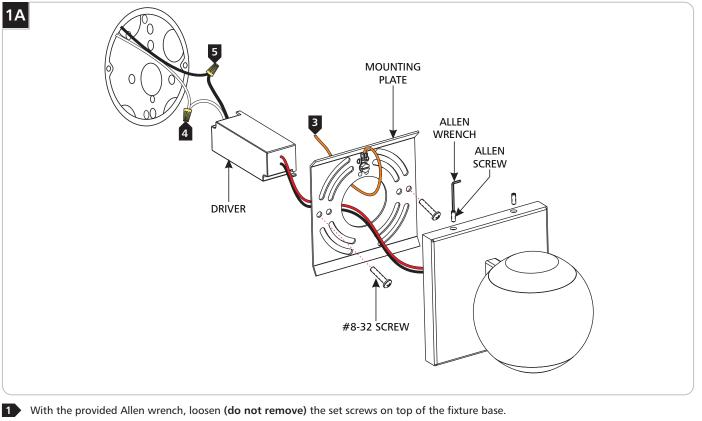
2 Remove the mounting plate from the back of the fixture.
