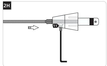
Firmly tighten the set screw on the conical connector.
