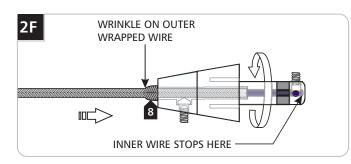
8 Keep pushing the coaxial cable into the connector while rotating the connector to ease feeding the inner wire into the tip of the connector. The outer wrapped wire will start wrinkling while being inserted another 1/2" into the connector.
