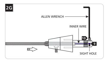
Dook into the sight hole on the top of the connector to make sure that the inner wire is contacting the end of the connector.
