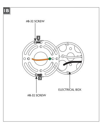
Install the mounting plate onto the electrical box with the two #8-32 screws provided.
