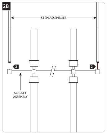
2 Feed the fixture wires through the stem assembly, then screw both stem assemblies onto the socket assembly.
