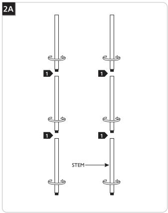
1 Determine the desired height of the fixture using the provided stems and assemble them by screwing them together.
