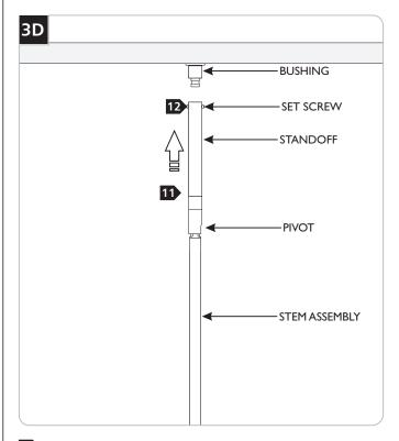
11 Lift the stem assembly up to the bushing
