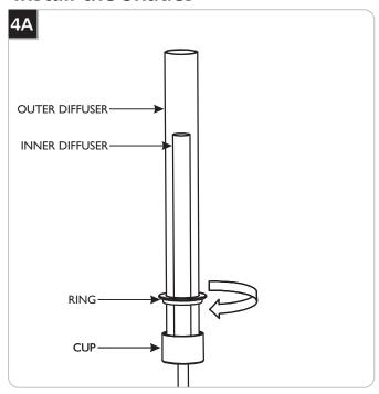
Insert the inner diffuser into the cup followed by the outer diffuser, then slide the ring over the outer diffuser and screw it into the cup to secure in place. Repeat for remaining diffusers.
