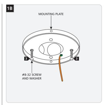
Secure the mounting plate to the electrical box with the #8-32 screws provided.
