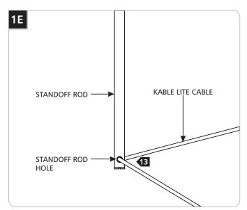
For each standoff rod, feed the Kable Lite cable coming from a turnbuckle through the insulated standoff rod hole into the other turnbuckle.
