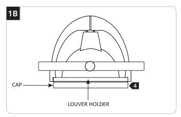
4 Screw the cap back onto the louver holder.
