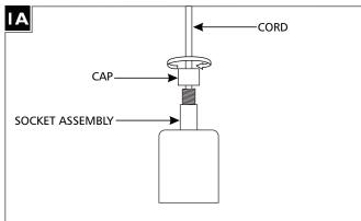
Unscrew fixture cap and remove the cap from the socket assembly and cord.
