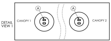
REPEAT STEPS 1-4 FOR BOTH CANOPIES. ORIENTATION MUST BE AS SHOWN IN DETAIL VIEW 1. TABS MARKED WITH A MUST BE IN LINE ON BOTH CANOPIES
