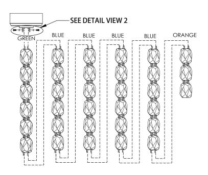
Each string of lights is identified by colored straps. Remove straps before installing. Connect sections as shown in the figure above. First, connect Green section to canopy, then attach Blue middle sections. At the end, attach Orange end section.
