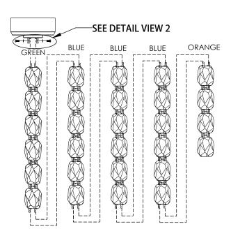
Each string of lights is identified by colored straps. Remove straps before installing. Connect sections as shown in the figure above. First, connect Green section to canopy, then attach Blue middle sections. At the end, attach Orange end section.
