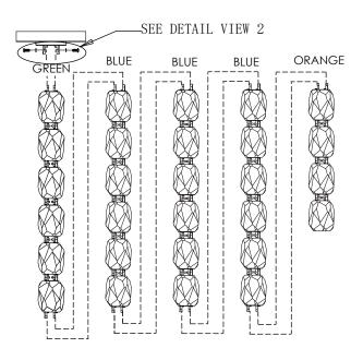
Each string of lights is identified by colored straps. Remove straps before installing. Connect sections as shown in the figure above. First, connect Green section to canopy, then attach Blue middle sections. At the end, attach Orange end section.
