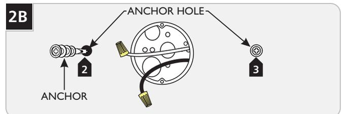
**2** Drill appropriate sized holes at the marked locations and install the anchor into the wall up to the threads.
