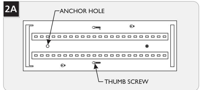
**1** Temporarily mount the fixture onto the mounting plate using the thumb screws, mark the anchor hole locations, and remove the back plate.
