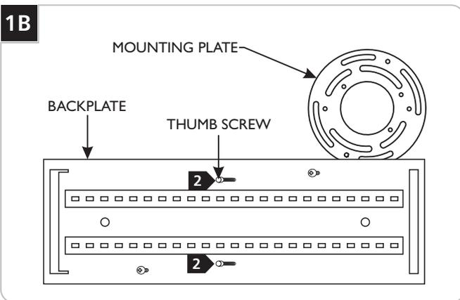
**2** Unscrew the two thumb screws to separate the mounting plate from the backplate.
