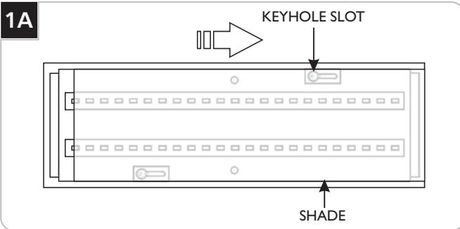
**1** Remove the shade by sliding it all the way over to release it from the keyhole slot, then carefully pull it straight out.
