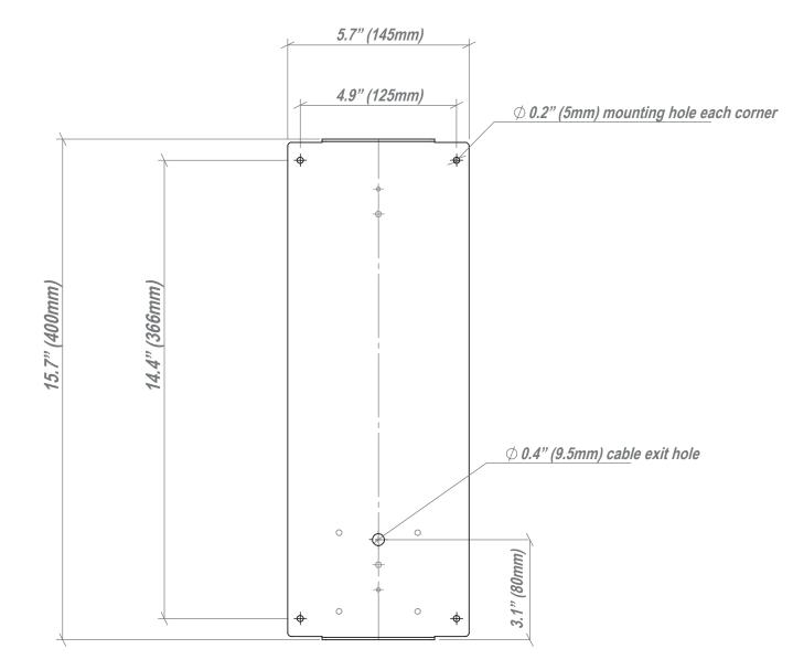
Backplates can be rotated 180 degrees- to allow cable exit to be positioned at top if required. Stated dimensions are for reference purposes only. Due to manufacturing tolerances, the actual dimensions of each product may differ to those stated.
