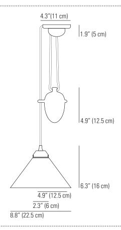
Cable length may be shortened upon installation. This will reduce both maximum & minimum dropand reduce the range of movement.
