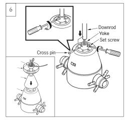
Slip downrod into motor housing yoke, aligning holes and Reinstall the cross pin. Insert cross pin through yoke and downrod and then fasten it with screwdriver. Pull the downrod up tight against the cross pin, and then evenly tighten the downrod set screws on motor housing yoke.
