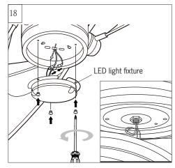
Connect white wire from fan to white wire from LED light fixture and then connect black (or blue) wire from fan to blue (or black) wire from LED light fixture.
