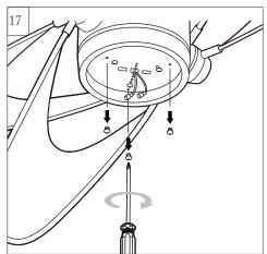
Remove 3 preassembled screw from the light pan. Save screws for later use.
