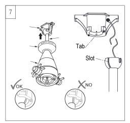
Install ball end of downrod into mounting bracket opening. Align (engage) slot on ball with tab on mounting bracket. **Warning:** Failure to align slot on ball with tab may result in serious injury. **Important:** If using the angle mount, make sure open end of mounting bracket is installed facing the higher point of the ceiling and make sure the ceiling angle is not steeper than 20°.
