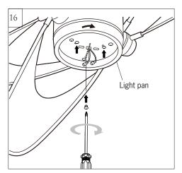
Place light pan over the lead wires and attach it onto the plate on motor. Align the keyhole slots on the light pan with the preassembled screws on the plate on motor. Twist clockwise till lock. Reinstall the screw removed in step 15. Tighten all screws securely.
