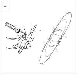
Align the screws holes in blade frame and the holes in the coupler and then fix the blades in the couplers with set screws provided.
