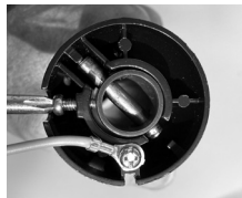
remove half-ball and stopper pin
