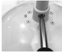
reinstall and tighten stopper screw
