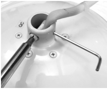
remove stopper screw and loosen hex screw
