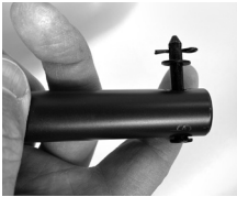
remove stopper pin, cotter pin and washer
