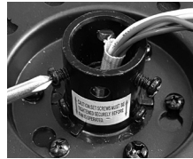
loosen screws on coupler
