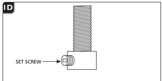
**6** Loosen (**Do Not Remove**) the set screw on each strain relief.
