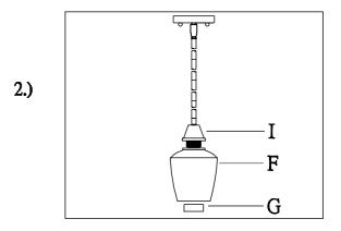
Step 2. Attached the glass (F) on the socket then secure by socket ring (G).
