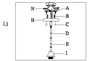
Step.1: Remove mounting bracket from fixture and install to electrical box
